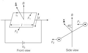
The thicker wire has a resistance R, then the other wire has a resistance 2R as the wires are of the same material but with cross-sections differing by a factor 2. Now, the force and hence, torque on first wire is given by
